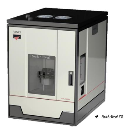
The presence of sulfur in oil reservoirs and / or oils plays an important role in issues related to oil exploration and refining. Rock-Eval 7S and Geoworks software make it **possible to analyze organic and mineral sulfur** in addition to hydrocarbons, CO and CO<sub>2</sub> and thus better understand the issues linked to oil exploration and exploitation.
